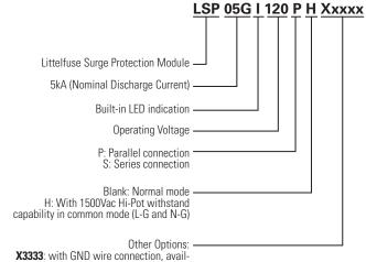
X3333: with GND wire connection, available for 240Vac and 277Vac rating with CE Marking for Class I earthed luminaire installation Wire Color: Line: Brown, Neutral: Blue, Ground/PE: Green with yellow stripe
