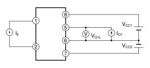
Fig.2 Test Circuit for O<sub>2</sub> High Level Output Voltage
