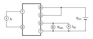
Fig.4 Test Circuit for O1 Leak Current
