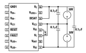
Figure 58.  $I_{\text{CL}}$  test circuit.
