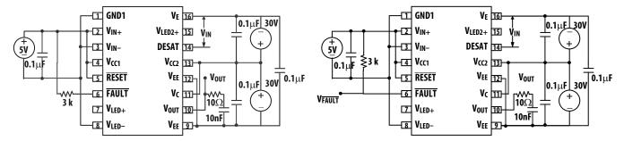
Figure 45. t<sub>DESAT</sub>(10%) test circuit.
