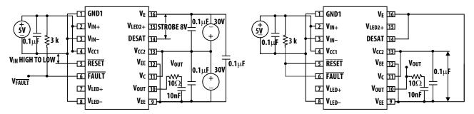
Figure 47. t<sub>RESET</sub>(FAULT) test circuit.
