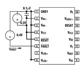
Figure 30. IFAULTH test circuit.
