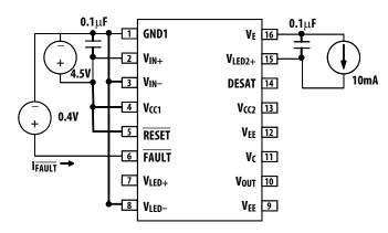
Figure 29. IFAULTL test circuit.
