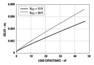
Figure 26. DESAT sense to 10% Vout delay vs. load capacitance.
