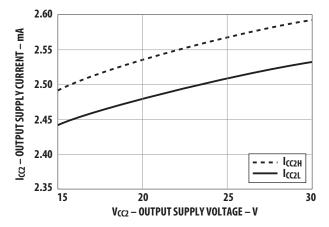
Figure 12. I<sub>CC2</sub> vs. V<sub>CC2</sub>.
