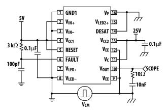
Figure 52. CMR test circuit, LED1 on.
