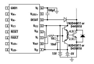
Figure 64. Output pull-down resistor.
