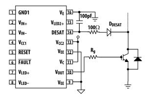
Figure 65. DESAT pin protection.
