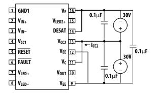
Figure 39. I<sub>CC2L</sub> test circuit.
