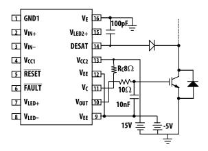
Figure 73. Use of RC to further limit I<sub>ON,PEAK</sub>.
