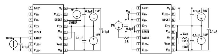
Figure 43. DESAT threshold test circuit.
