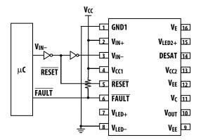
Figure 72d. Safe hardware reset for inverting input configuration (automatically resets for every V<sub>IN</sub>. input).
