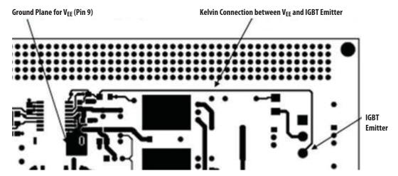
Figure 77c. Kelvin Connection between VEE and IGBT Emitter
