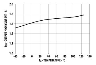
Figure 3.  $I_{OH}$  vs. temperature.
