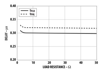
Figure 22. Propagation delay vs. load resistance.
