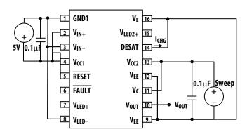
Figure 42. UVLO threshold test circuit.
