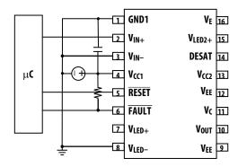
Figure 67. Typical input configuration, noninverting.
