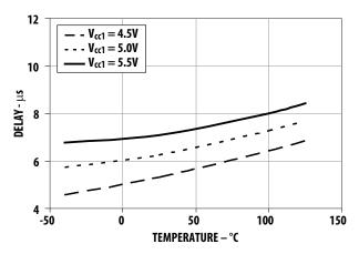
Figure 28. RESET to high level fault signal delay vs. temperature.
