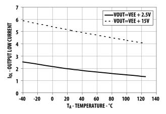
Figure 4.  $I_{OL}$  vs. temperature.
