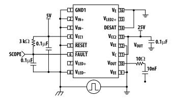
Figure 49. CMR test circuit, LED2 off.
