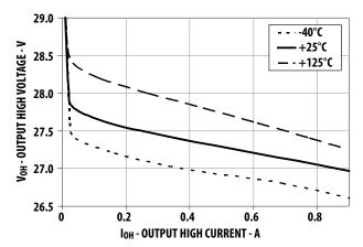
Figure 8. V<sub>OH</sub> vs. I<sub>OH</sub>.
