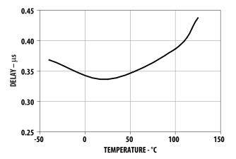
Figure 23. DESAT sense to 90% Vout delay vs. temperature.
