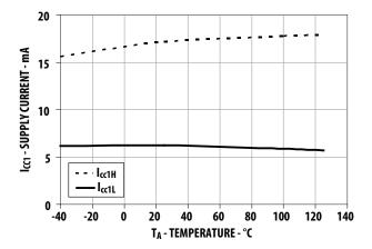
Figure 10. I<sub>CC1</sub> vs. temperature.
