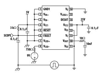
Figure 50. CMR test circuit, LED2 on.
