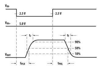
Figure 54.  $\rm V_{OUT}$  propagation delay waveforms, inverting configuration.
