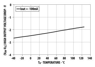
Figure 6. V<sub>OH</sub> vs. Temperature.
