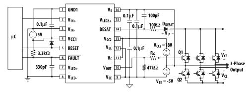
Figure 61. Recommended application circuit.
