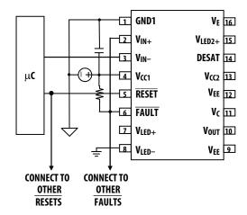
Figure 70. Global-shutdown, global reset configuration.
