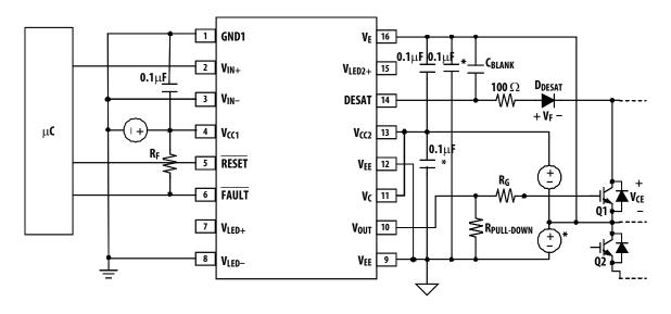
Typical de-saturation protected gate drive circuit, non-inverting.
