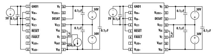
Figure 56. I<sub>CH</sub> test circuit.
