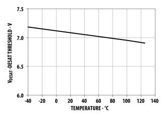
Figure 16. DESAT threshold vs. temperature.
