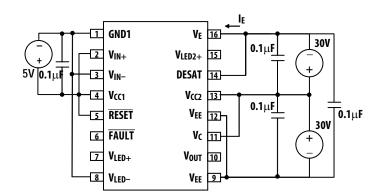
Figure 59.  $I_{EH}$  test circuit.
