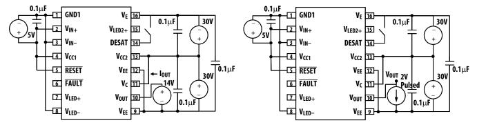
Figure 33. l<sub>OLF</sub> test circuit.
