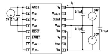
Figure 60.  $I_{\text{EL}}$  test circuit.
