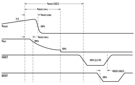
Figure 55. Desat,  $V_{\text{OUT}}$ , fault, reset delay waveforms.
