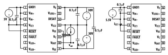
Figure 35. V<sub>OL</sub> test circuit.
