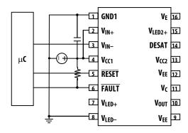
Figure 68. Typical Input Configuration, Inverting.
