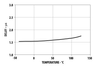
Figure 24. DESAT sense to 10% Vout delay vs. temperature.
