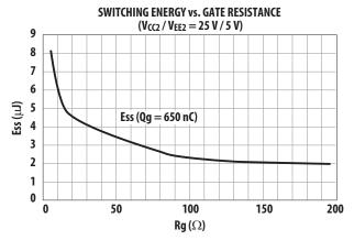
Figure 76. Switching energy plot for calculating average P<sub>switch</sub> (for ACPL-38JT output driving an IGBT rated at 600 V/100 A).
