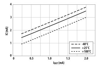
Figure 15. I<sub>C</sub> vs. I<sub>OUT</sub>.
