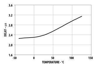
Figure 25. DESAT sense to low level fault signal delay vs. temperature.
