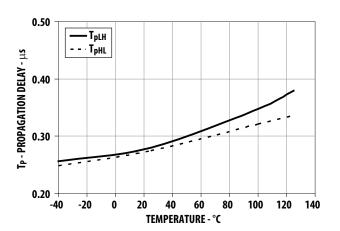
Figure 17. Propagation delay vs. temperature.
