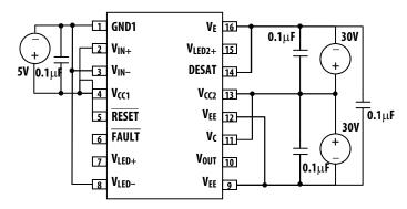
Figure 38.  $I_{\text{CC2H}}$  test circuit.
