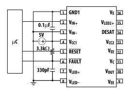
Figure 66. FAULT Pin CMR protection.
