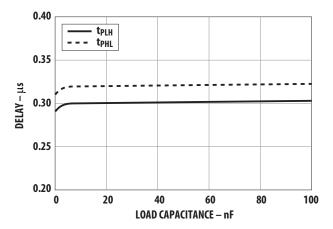
Figure 21. Propagation delay vs. load capacitance.
