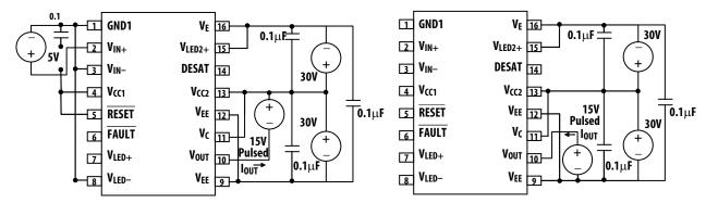
Figure 31. I<sub>OH</sub> pulsed test circuit.
