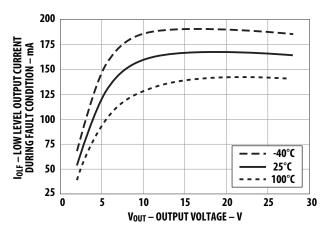
Figure 5. I<sub>OLF</sub> vs. V<sub>OUT</sub>.
