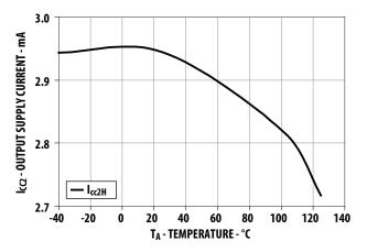
Figure 11.  $I_{CC2}$  vs. temperature.
