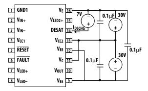
Figure 41. I<sub>DSCHG</sub> test circuit.
