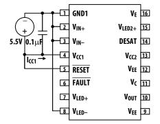
Figure 37. I<sub>CC1L</sub> test circuit.
