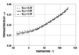
Figure 19.  $V_{\text{IN}}$  to high propagation delay vs. temperature.
