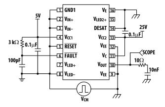
Figure 51. CMR test circuit, LED1 off.
