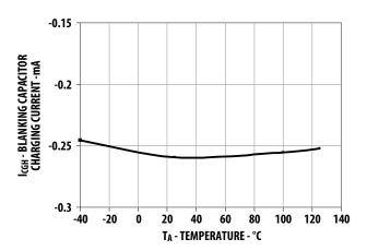
Figure 13. I<sub>CHG</sub> vs. temperature.
