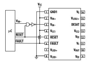
Figure 72c. Safe hardware reset for inverting input configuration.
