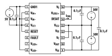
Figure 40. I<sub>CHG</sub> pulsed test circuit.
