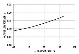
Figure 7. V<sub>OL</sub> vs. Temperature.
