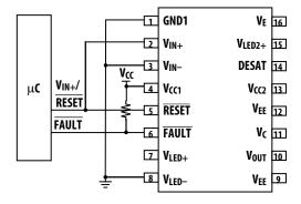
Figure 72a. Safe hardware reset for non-inverting input configuration (automatically resets for every  $V_{\rm IN+}$  input).
