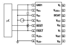
Figure 69. Local shutdown, local reset configuration.
