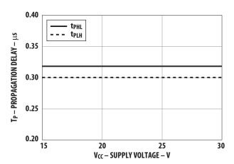
Figure 18. Propagation delay vs. supply voltage.
