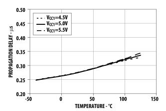
Figure 20.  $\ensuremath{V_{\text{IN}}}$  to low propagation delay vs. temperature.
