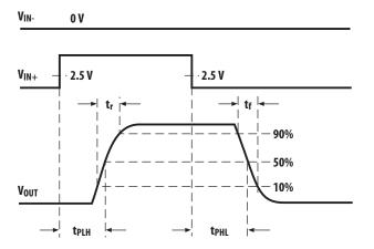
Figure 53.  $V_{\text{OUT}}$  propagation delay waveforms, noninverting configuration.
