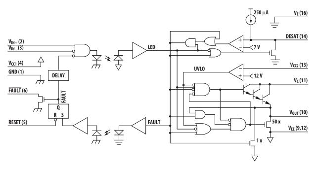
Figure 63. Behavioral circuit schematic
