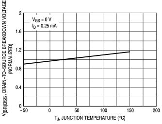
Figure 5. Breakdown Voltage Variation
