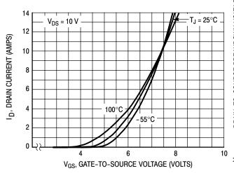
Figure 4. Transfer Characteristics
