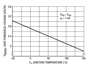
Figure 3. Gate-Threshold Voltage Variation With Temperature
