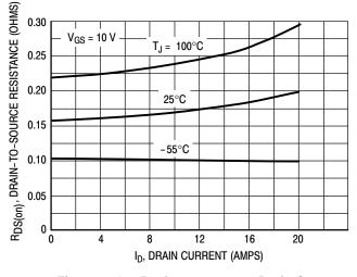
Figure 6. On-Resistance versus Drain Current
