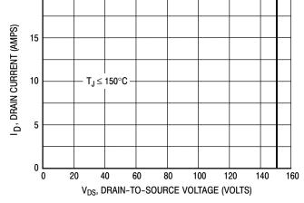
Figure 9. Maximum Rated Switching Safe Operating Area
